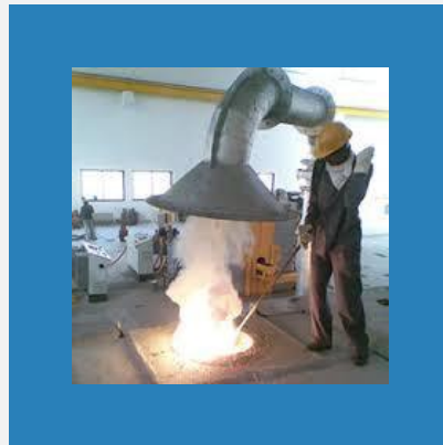
Fume Extraction System
